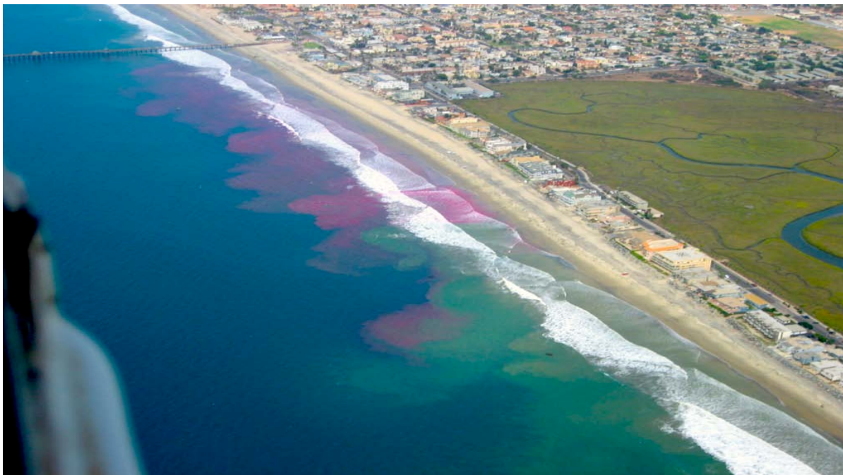
Figure 5: Aerial photograph during the IB09 plume experiment with South swell. Dye injected continuously near the shoreline was advected northward (toward the image top) by the breaking-wave driven alongshore current. A fixed array of instruments (downcoast of the Imperial Beach Pier, upper left) spanned from the shoreline to about 5m depth. The jetski sampling pattern was similar to Huntington Beach (figure 1) but spanned several km of dye plume (figure 6).
