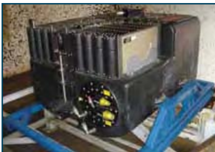
Figure 7 IAFS Combo-Pak - Instrumented and Mounted On Ballistic Test Stand
