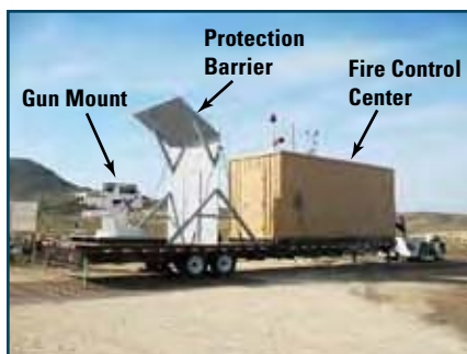
Figure 9 Portable Fire Control Center (The War Wagon)
