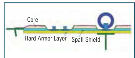
Figure 3 Selected Floor Configuration with Integral Armor
