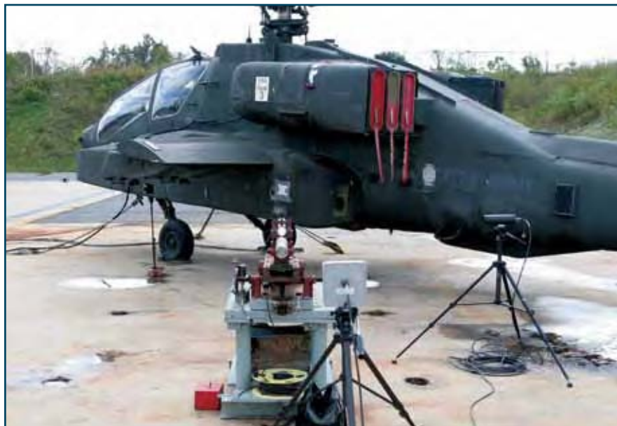
Figure 8 IAFS Combo-Pak Testing - Installed In AH-64D GTV
