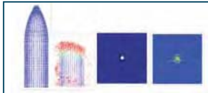
Figure 5 Predictions of Damage to Penetrator, CMC Layer, and Ceramic Layer
