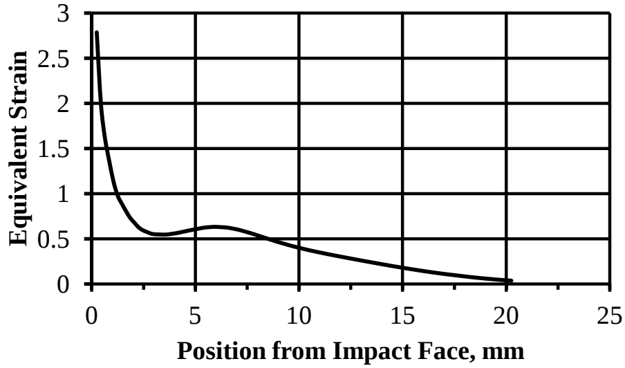
Figure 14. Equivalent strain values from EPIC simulations along the center-line of the tantalum Taylor Impact specimen.
