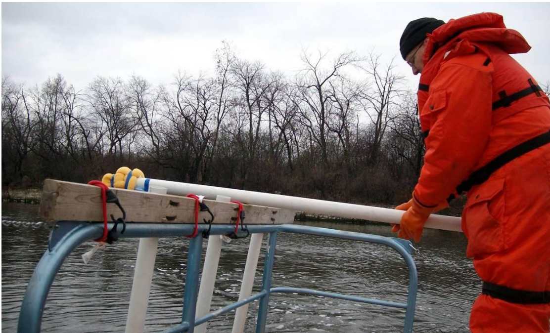
Figure 13. Preparing for canal wall touch point current with pole and sponge electrode.
