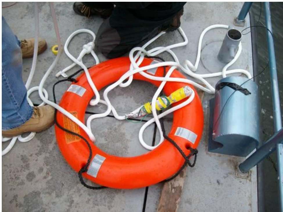
Figure 15. Simulated PIW with input electrode and life ring.
