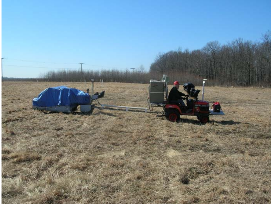
Figure 1. Demonstrator's system, EM61 MKII/towed array.
