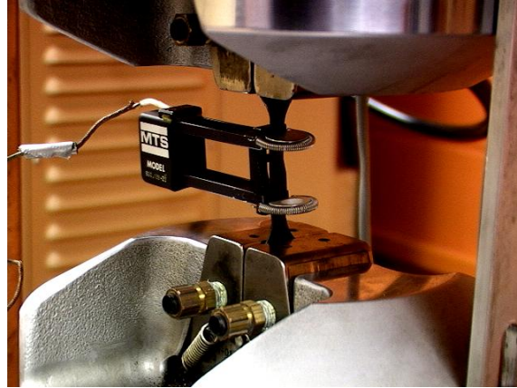
Figure 4. Coupon with Extensometer
