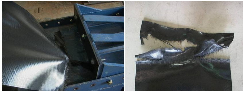
Figure 107. Sample 28 (Failure/Post-Test Damage)
