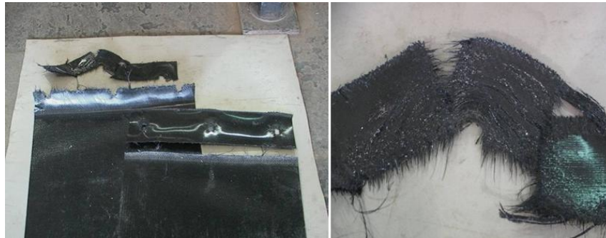
Figure 93. Sample 20 (Failure/Post-Test Damage)
