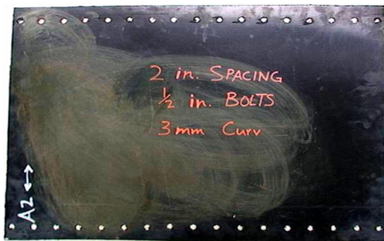
Figure 17. Mechanical Connection (Sample A2 – Pre-Test)
