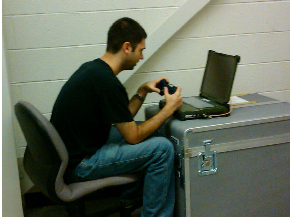
Figure 1: The current method to control a UGV is with a laptop using rate-controlled teleoperation.
