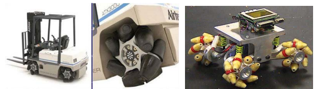
Fig. 3 Examples of vehicles using Mecanum wheels (from [7] and [8])
