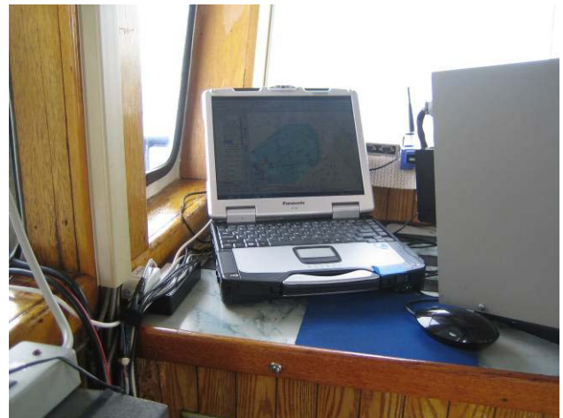
Figure 1. AIS receiver, router, WiFi system, and ruggedized notebook computer are shown as they were installed on the bridge of the R/V Sproul during Leg II of SOCAL 10.
