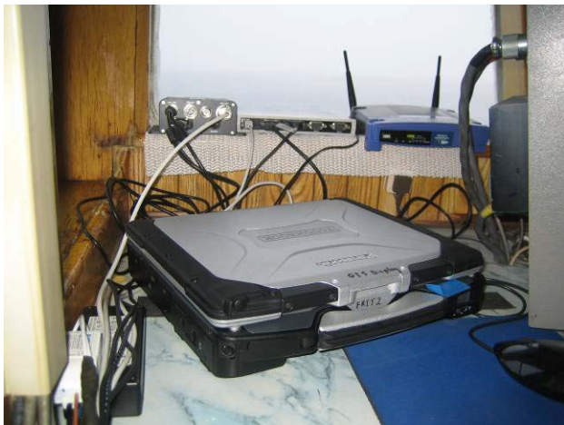
Figure 1. AIS receiver, router, WiFi system, and ruggedized notebook computer are shown as they were installed on the bridge of the R/V Sproul during Leg II of SOCAL 10.
