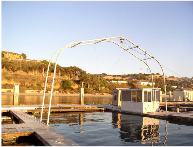
Figure 2. Picture of the floating test site. The overhead frame supports two cameras that look down on the 30x60 ft pen. The control hut, from which operations are run, is on the opposite side of the camera frame. Station B, behind which the sound emitting transducer hangs, is the at the mid-point of the far end of the pen.
