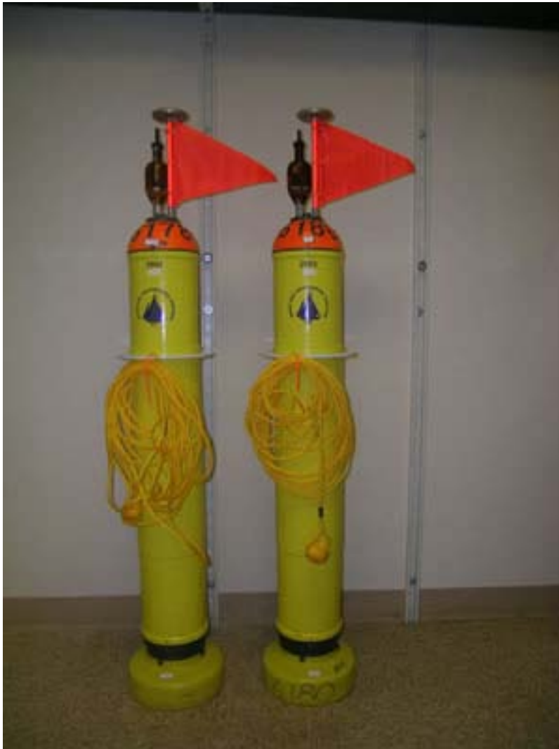
Figure 2: Photo of APEX Profilers with installed DMON and 3-channel hydrophone assembly (top end cap to left of flag). Profilers were modified to enable post-experiment recovery, including addition of Iridium 2-way satellite communications.
