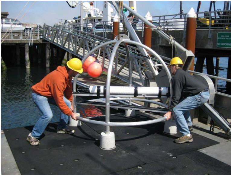
Figure 2. Configuration of a passive acoustic sensor within its mooring frame. See Figure 1 for the distribution of four of these sensors across the study area.
