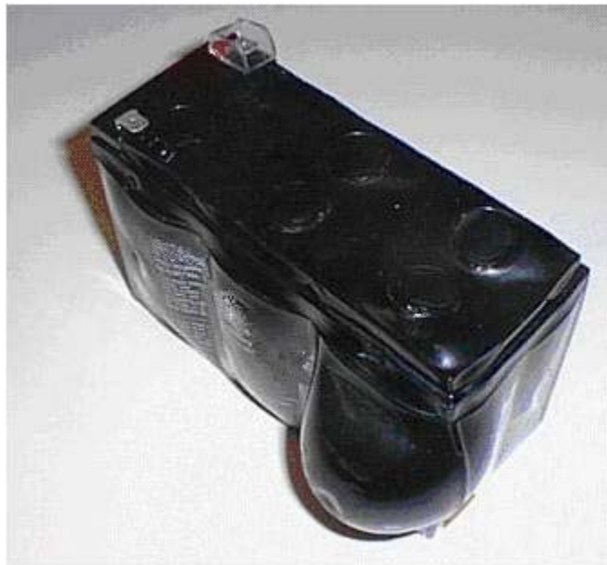
Figure 3. Battery deformation that resulted from a thermal runaway. [5]
