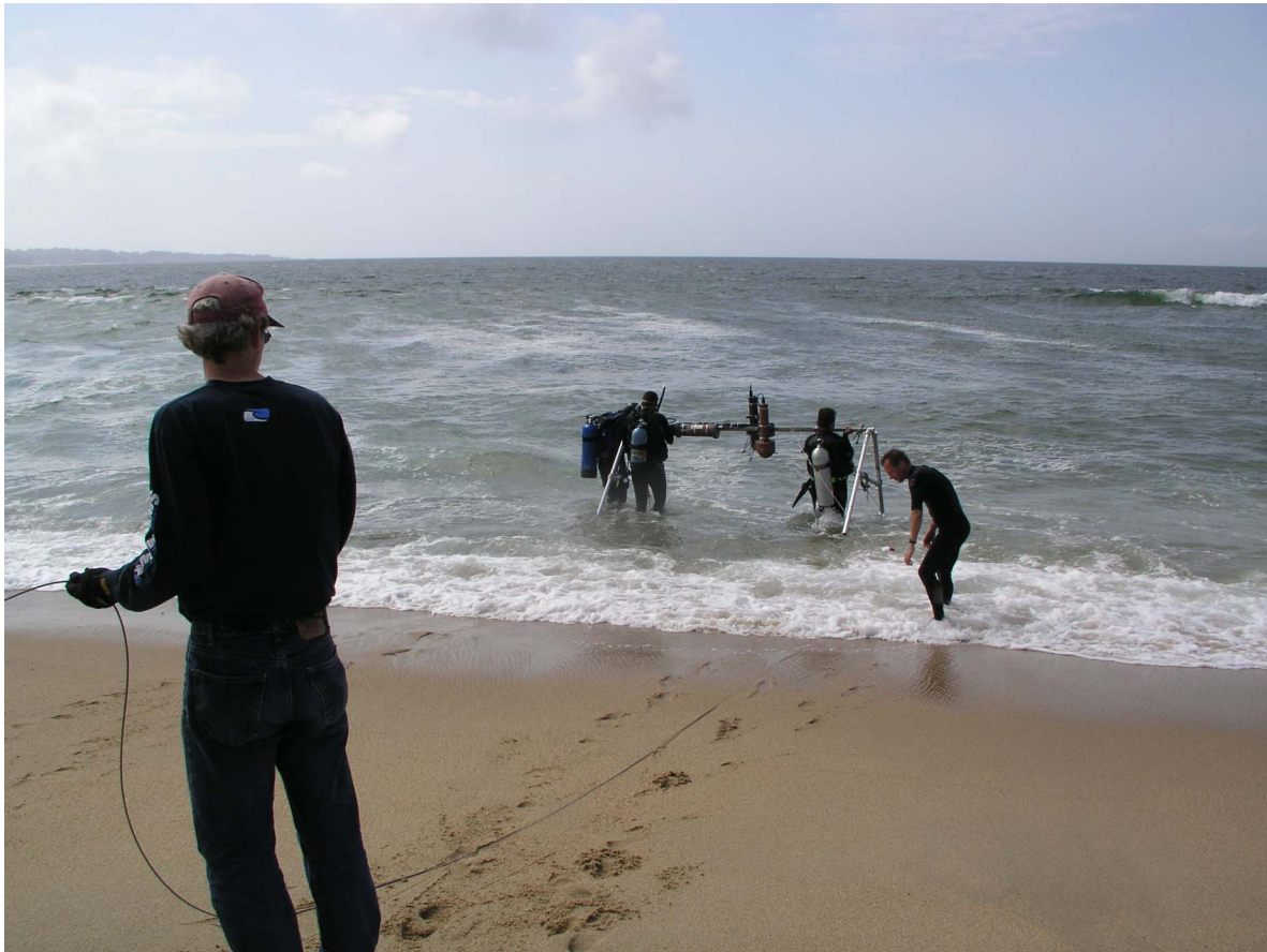
Figure (1) Deploying the Bottom Boundary Layer frame into the rip channel during RCEX, with the temporary side supports in place. The frame was supported within the channel by two poles that had previously been jetted in. The BCDVSP and scanned altimeter can be seen near the center of the cross-shore support beam
