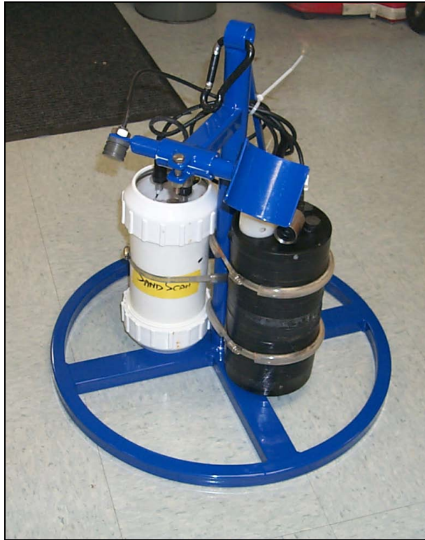
Figure 2: The Sand Scan acoustic sensor consists of a broadband acoustic transducer, a small grey cylinder shown here on a movable arm at the upper left of the instrument. The white pressure case contains the electronics necessary to transmit a sequence of 200-microsecond pulses at several discrete frequencies between ca 0.16 and 0.40 MHz, receive the echoes from a small area on the seabed, and store digital representations of the received bottom reverberation waveforms. The black cylinder contains batteries. For scale, the tiles on the lab floor were 1 foot on each side.
