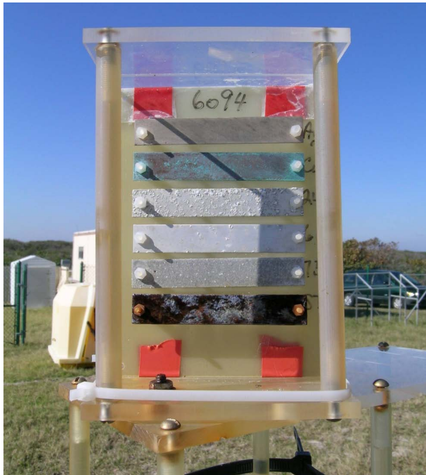
Figure A15. Test rack at Kennedy Space Center beach site, 90 days.
