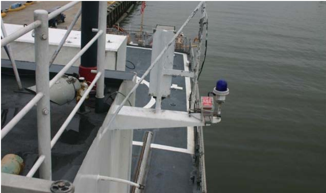
Figure A1. Test rack on USCGC Bear; above deck.
