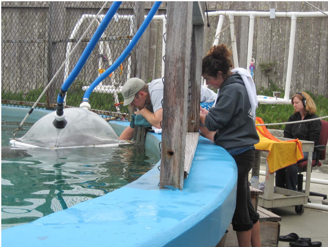
Figure 1. Photograph taken during one experimental session showing the equipment set-up which includes the metabolic hood, the dolphin stationed under the metabolic hood, the acoustic recording equipment and operator, the dolphin trainer, and the assistant taking notes and recording respirations. During the trial the dolphin is acoustically monitored and all respirations are recorded during each of the three periods.
