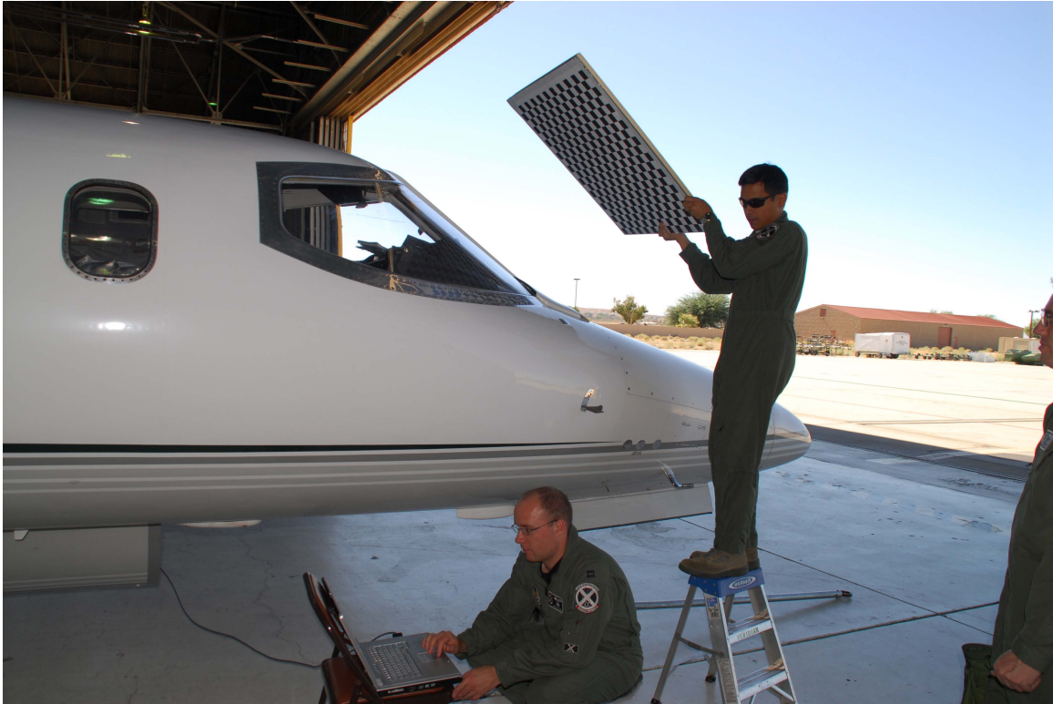
Figure 5.14: Collecting camera calibration images. This process was more difficult than the average laboratory setting, flexing in the original board caused errors in the model.
