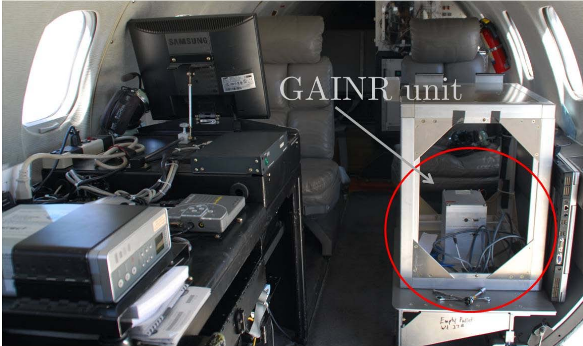
Figure 5.12: Truth collection device installed on the project LJ-25. A similar unit was installed in the nose of the T-38.
