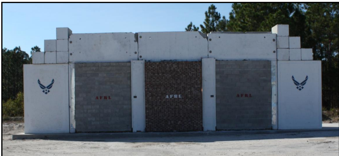
Figure 5. Test panels ready for dynamic loading
