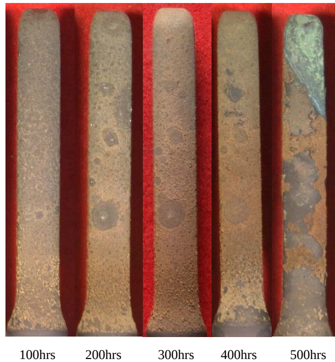
Figure 3-31. The effects of DiEGME/Jet A blended baseline on the leading edge of test bar 11C (PWA 663/PWA 73) after hot corrosion testing for 100, 200, 300, 400 and 500 hours at 1600°F with 3.5ppm salt.
