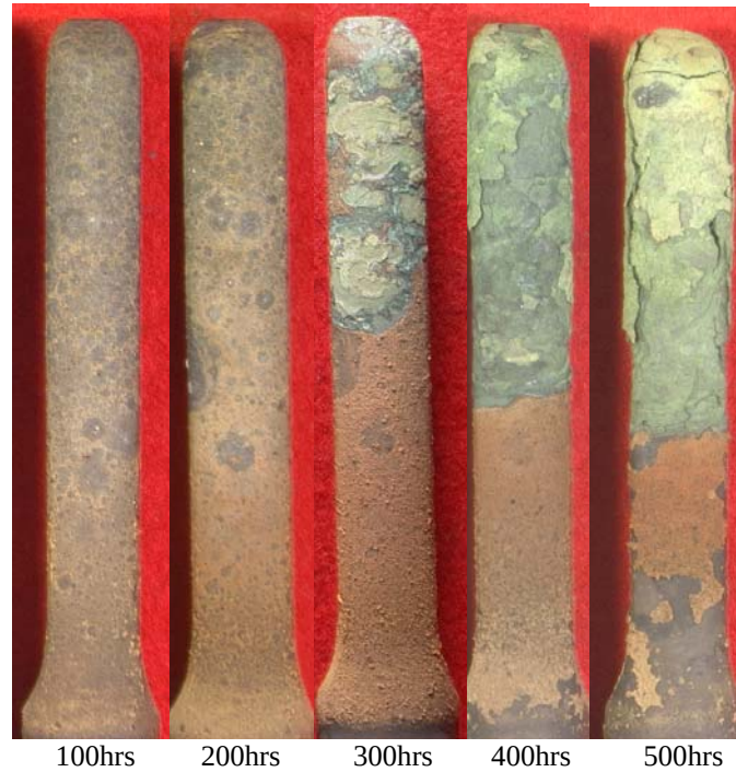
Figure 3-33. The effects of DiEGME/Jet A blended baseline on the leading edge of test bar 6C (PWA 655/PWA 73) after corrosion testing for 100, 200, 300, 400 and 500 hours at 1600°F with 3.5 ppm salt.
