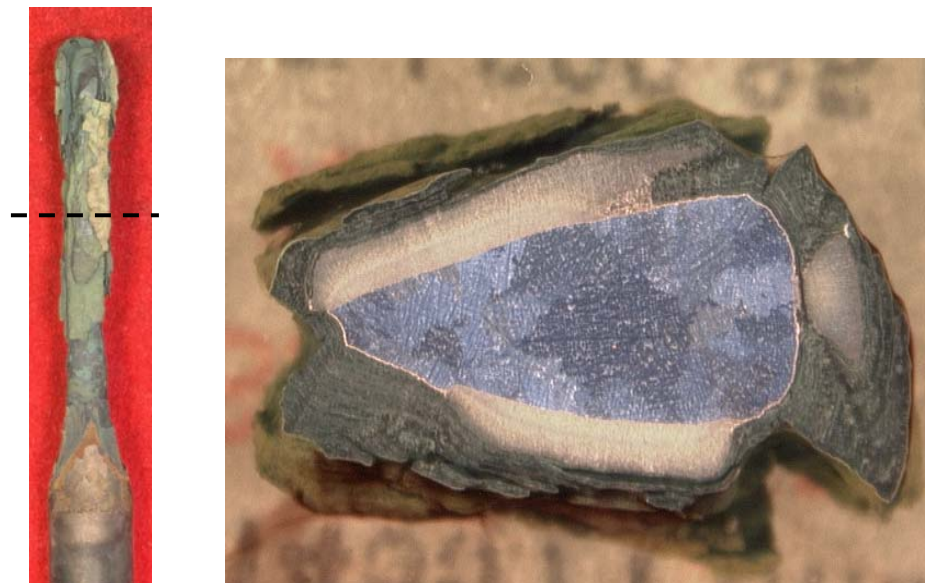
Figure 3-52. Test bar 9D (2043F) showing the effects of the TriEGME/Jet A blend on PWA 1455/Uncoated after corrosion testing for 500.85 hours at 1600°F with 3.5 ppm salt.
