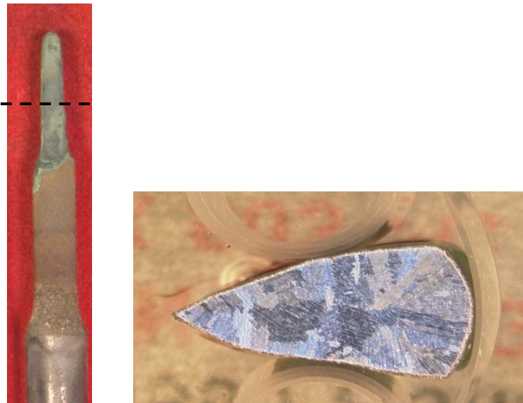
Figure 3-48. Test bar 12D (2158G) showing the effects of the TriEGME/Jet A blend on PWA 655/Uncoated after corrosion testing for 500.85 hours at 1600°F with 3.5 ppm salt.
