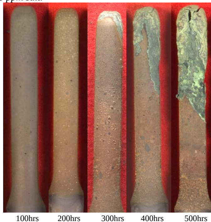
Figure 3-34. The effects of TriEGME/Jet A blended mixture on the leading edge of test bar 8D (PWA 655/PWA 73) after corrosion testing for 100, 200, 300, 400 and 500 hours at 1600°F with 3.5 ppm salt.
