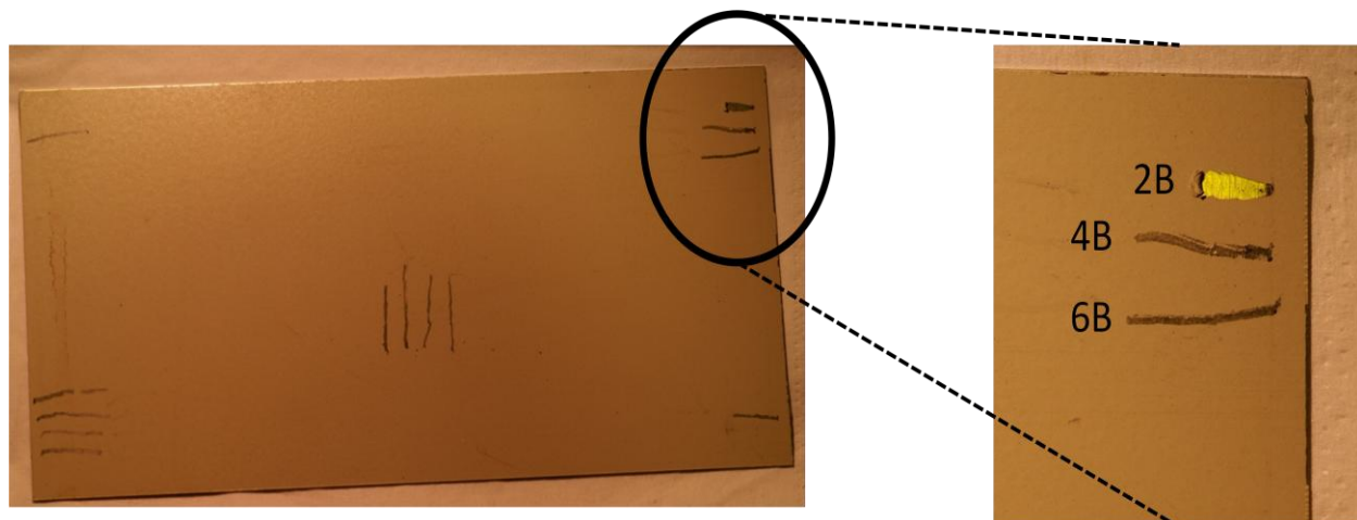
Figure 15. Old panel exposed to condensed vapors from 0.08 vol% DiEGME in the fuel with the pencil hardness measurements shown.
