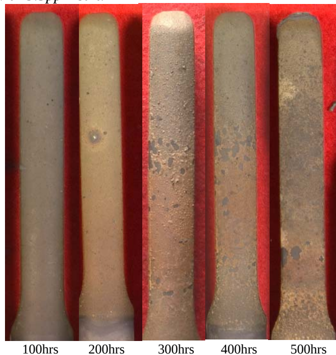
Figure 3-32. The effects of TriEGME/Jet A blended mixture on the leading edge of test bar 11D (PWA 663/PWA 73) after hot corrosion testing for 100, 200, 300, 400 and 500 hours at 1600°F with 3.5ppm salt.
