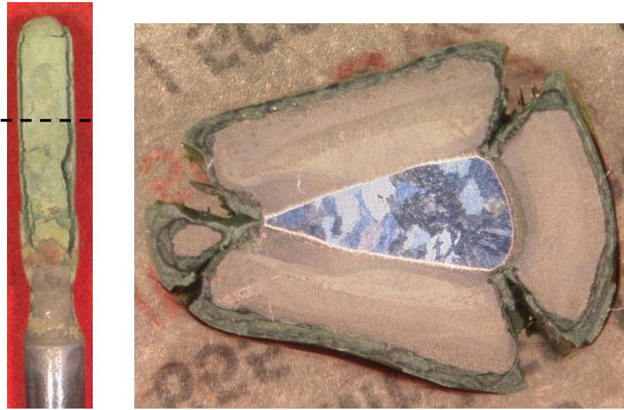
Figure 3-47. Test bar 12C (2158P) showing the effects of the DiEGME/Jet A baseline blend on PWA 655/Uncoated after corrosion testing for 500 hours at 1600°F with 3.5 ppm salt.
