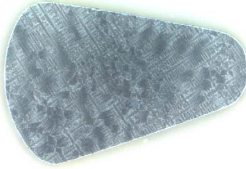
TriEGME – E-Bar S/N 1740S (Uncoated PWA 1484)
