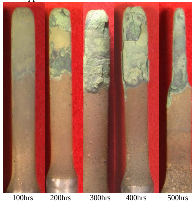
Figure 3-35. The effects of DiEGME/Jet A blended baseline on the leading edge of test bar 12C (PWA 655/Uncoated) after corrosion testing for 100, 200, 300, 400 and 500 hours at 1600°F with 3.5 ppm salt.
