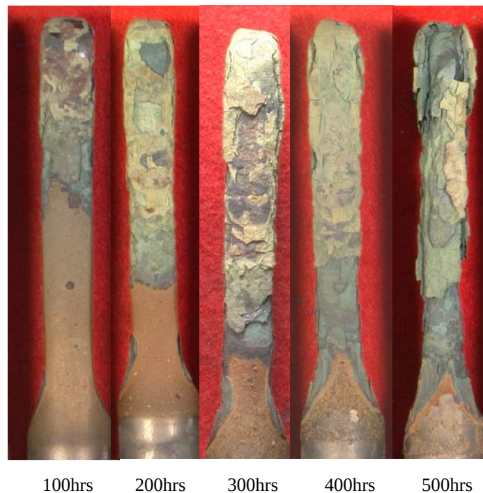
Figure 3-38. The effects of TriEGME/Jet A blended mixture on the leading edge of test bar 9D (PWA 1455/Uncoated) after corrosion testing for 100, 200, 300, 400 and 500 hours at 1600°F with 3.5 ppm salt.
