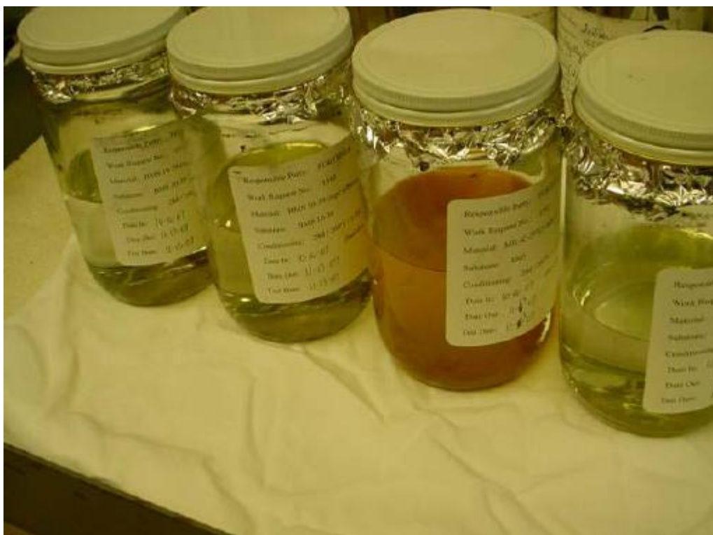
Figure 3. Fuel Discoloration of 1.5 times TriEGME after aging AMS-C-27725 polyurethane coating specimens.
