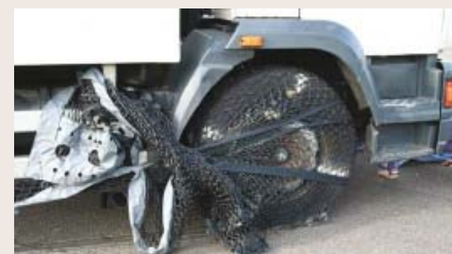
The M2 Vehicle Lightweight Arresting Device with Single Net Solution and Remote Deployment Device effectively stops a vehicle by entangling its tire.
