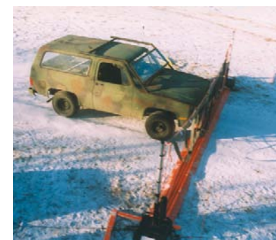
Portable Vehicle Arresting Barriers can effectively stop a vehicle, potentially enabling the capture of the driver. General Dynamics Corporation Photos
