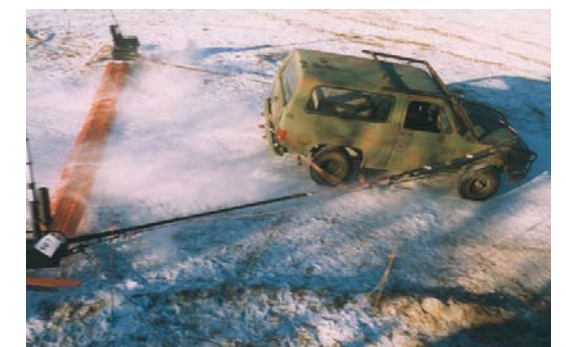
Portable Vehicle Arresting Barriers can effectively stop a vehicle, potentially enabling the capture of the driver. General Dynamics Corporation Photos
