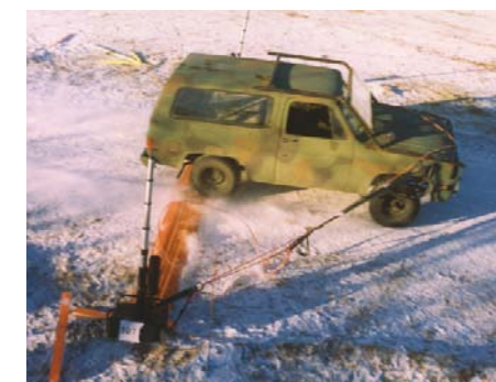
Portable Vehicle Arresting Barriers can effectively stop a vehicle, potentially enabling the capture of the driver. General Dynamics Corporation Photos
