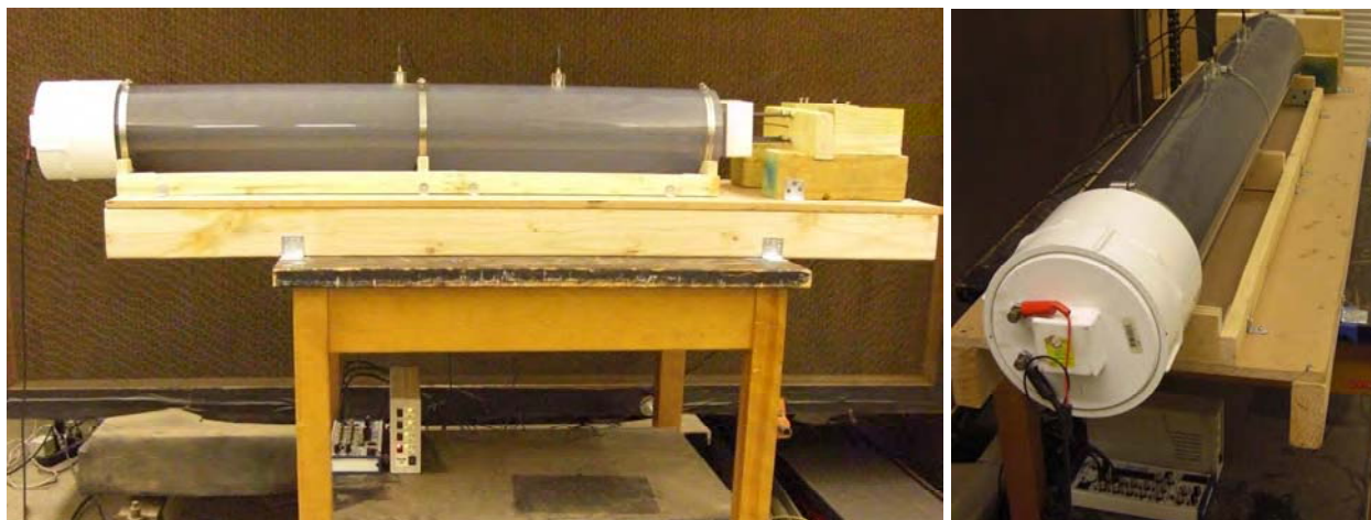
Figure 3: Photographs of blast tube for testing burst membrane prototypes. Side view ( left ) and view from end containing explosive charge ( right ).
