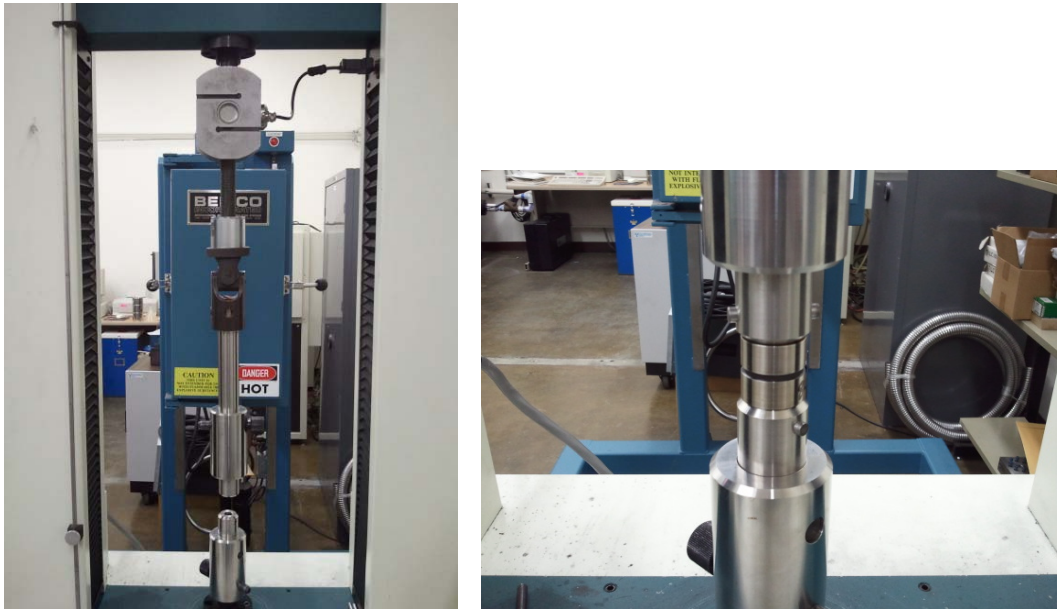
Figure 13: Custom designed load fixture for interlaminar tensile tests.
