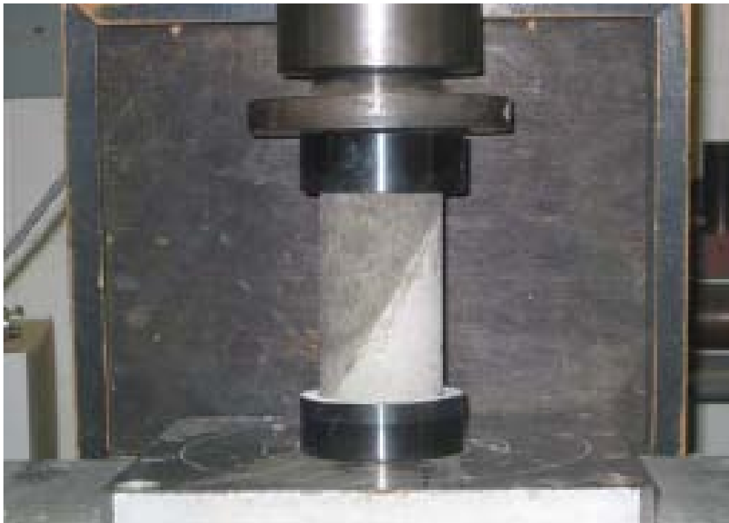
Figure 6. Slant shear sample undergoing test.
