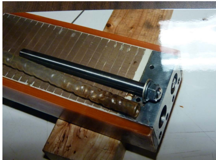
Figure 4. Bender bar with broken stress rod.
