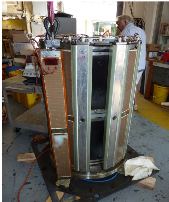
Figure 6. Installing bender bar S/N 016 as an inactive stave.
