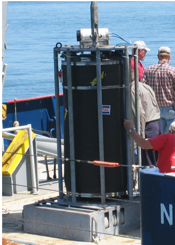
Figure 3. HX-554 projector configured as a dipping source.
