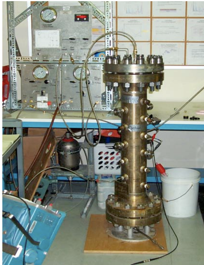
Fig. 1. The pressure vessel used for simulating the hydrostatic pressure at ocean depths up to 300 m is shown. The present acoustic resonator apparatus can be operated within this pressure vessel to investigate the hypothesis that trapped crevice gas controls the low frequency sound speed in water-saturated sand sediments.
