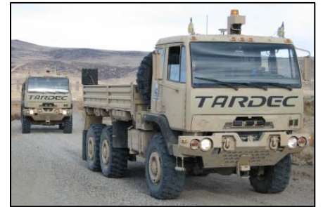
Tactical wheeled vehicles equipped with Convoy Active Safety Technology (CAST)
