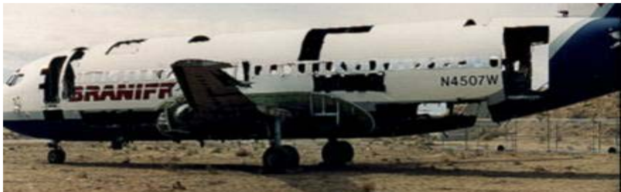
Figure 27-42: Cut-Outs Show where Fuselage Structure was Harvested from WFU Airframes.
