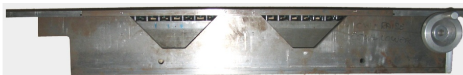
Figure 11-5: Side View of Mechanical Pillowing Simulator.
