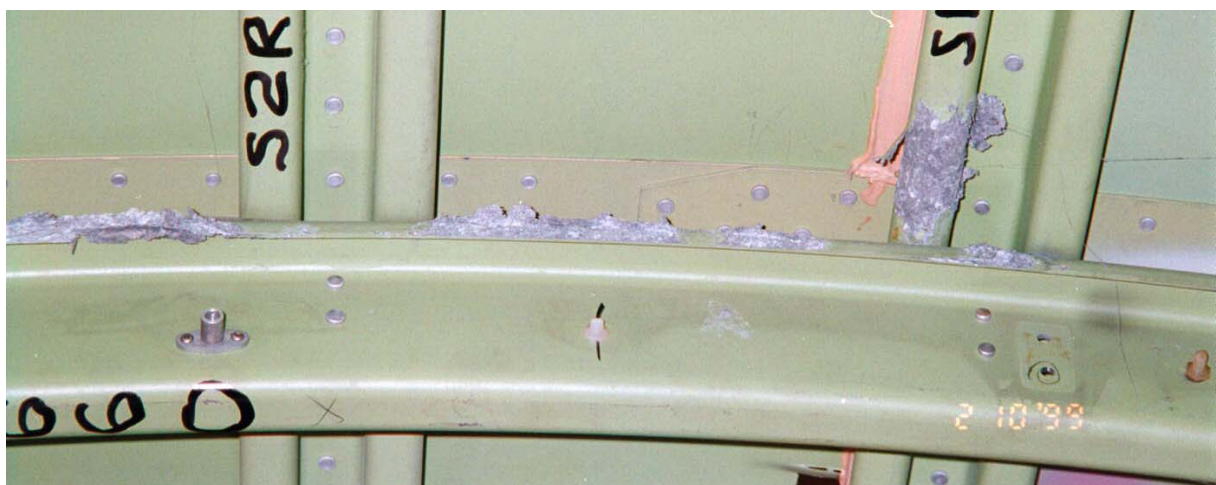
Figure 27-43: Stringer and Frame Corrosion in the Crown of a Stored Fuselage Due to Moisture Remaining in Insulation Blankets (Removed).
