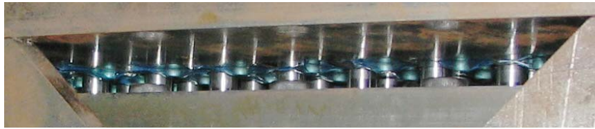
Figure 11-6: Close-Up Side-View of Pin Contact with Underside of Skin Sheet
