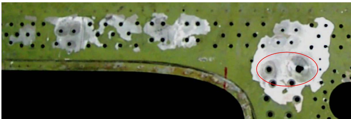
Figure 27-14: Upper Wing Skin with Exfoliation Corrosion Damage at Fastener Holes.
