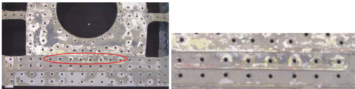
Figure 27-40: A 0.080 Inch (2.03 mm) Thick Shim In-Situ (left, circled), Enlarged (right).
