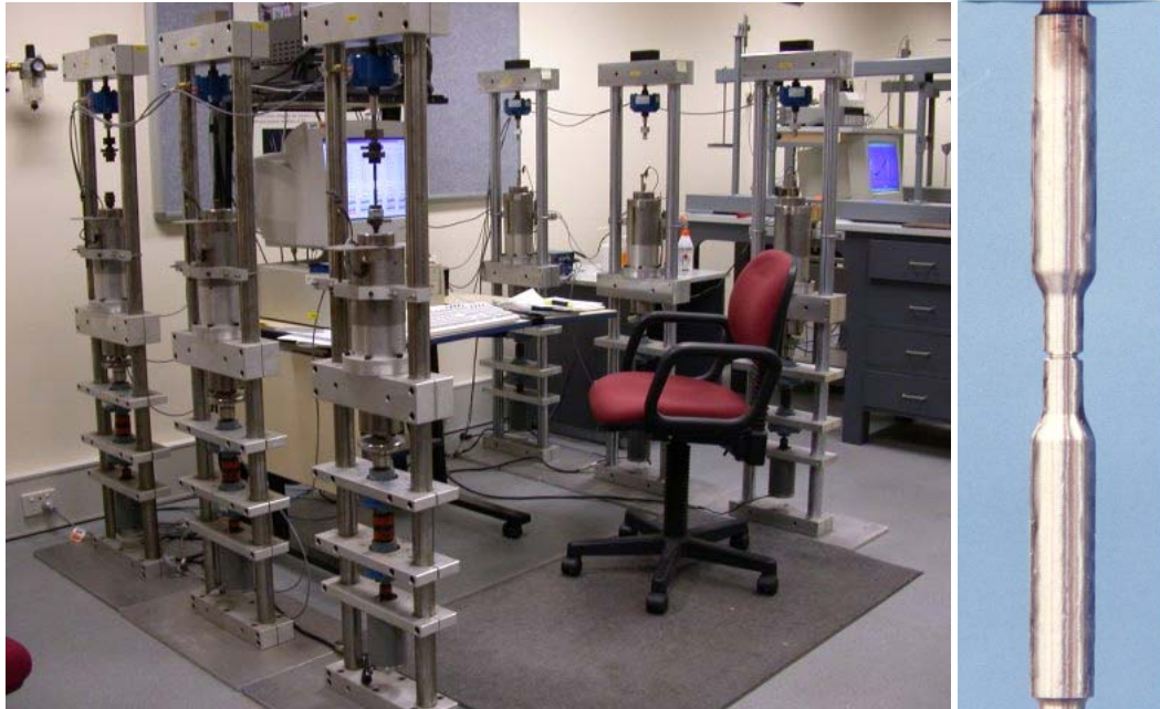
Figure 20-5: Slow Strain Rate Tensile (SSRT) Test Rigs and Example Test Specimen.
