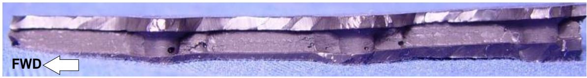
(a) Side view of replica from a fractured skin edge showing fracture surface.
