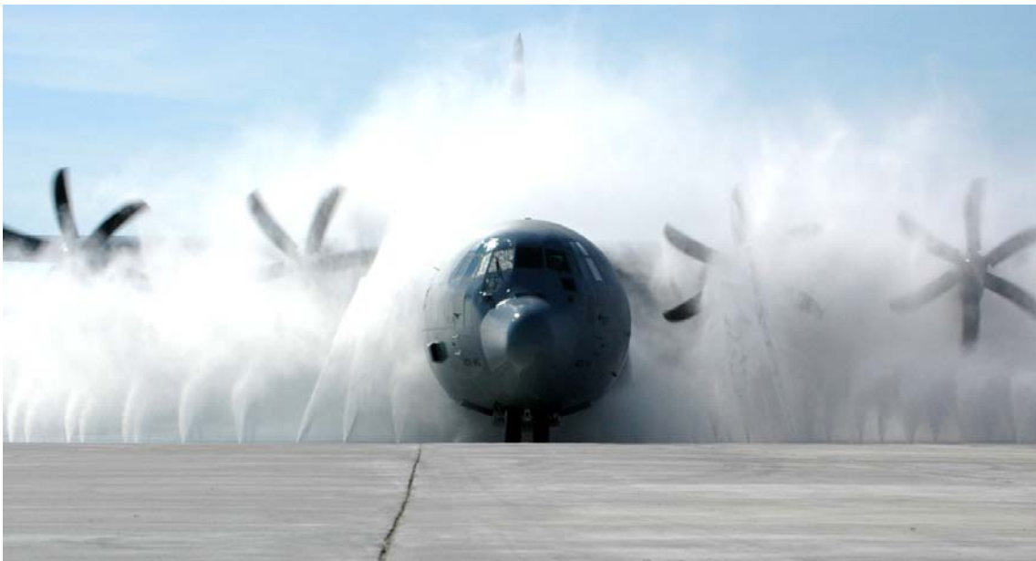
Figure 26-1: A C-130J Hercules is Cleaned Up in the New “Bird-Bath” System at Keesler Air Force Base, Biloxi, Mississippi. Aircraft from the Air Force Reserve fly many hours over the Gulf of Mexico. Salt and moisture could lead to corrosion if aircraft are not kept clean. (U.S. Air Force photo / Tech Sgt. Jame Pritchett).
