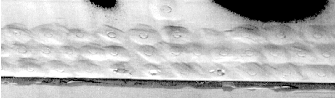
Figure 27-11: Exterior Spot Grinding.
