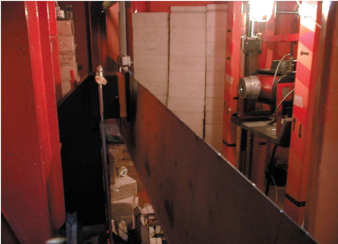
Figure 22-7: Mi-8 Type Rotor Blade Undergoing X-Ray Radiography.
