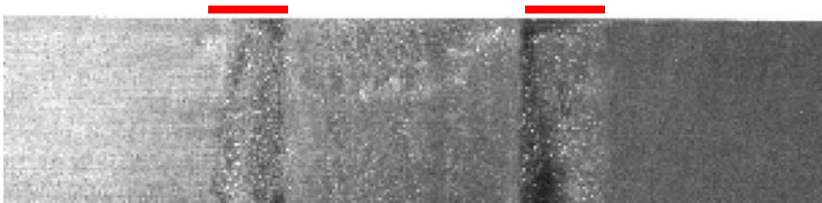
(b) Outer surface showing exfoliation corrosion (ASTM G-34).
