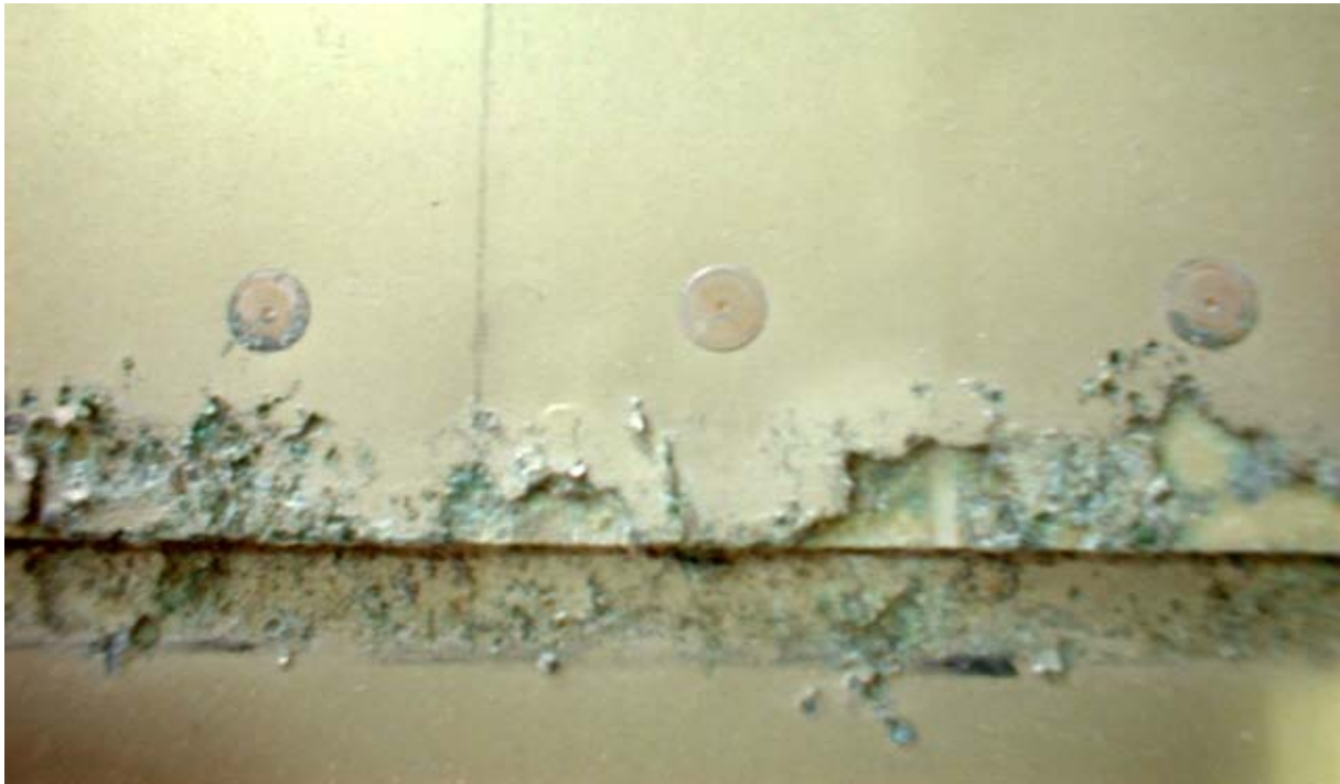
Figure 27-22: Corrosion Damage on Outer Surface of Glare Lap Joint.
