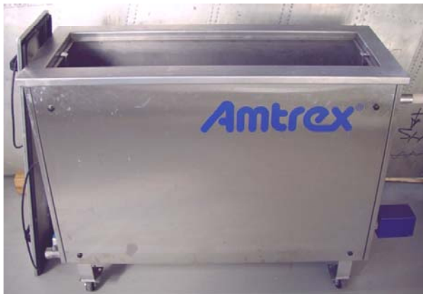
Figure 27-32: Ultrasonic Immersion Corrosion Cleaning Tank.
