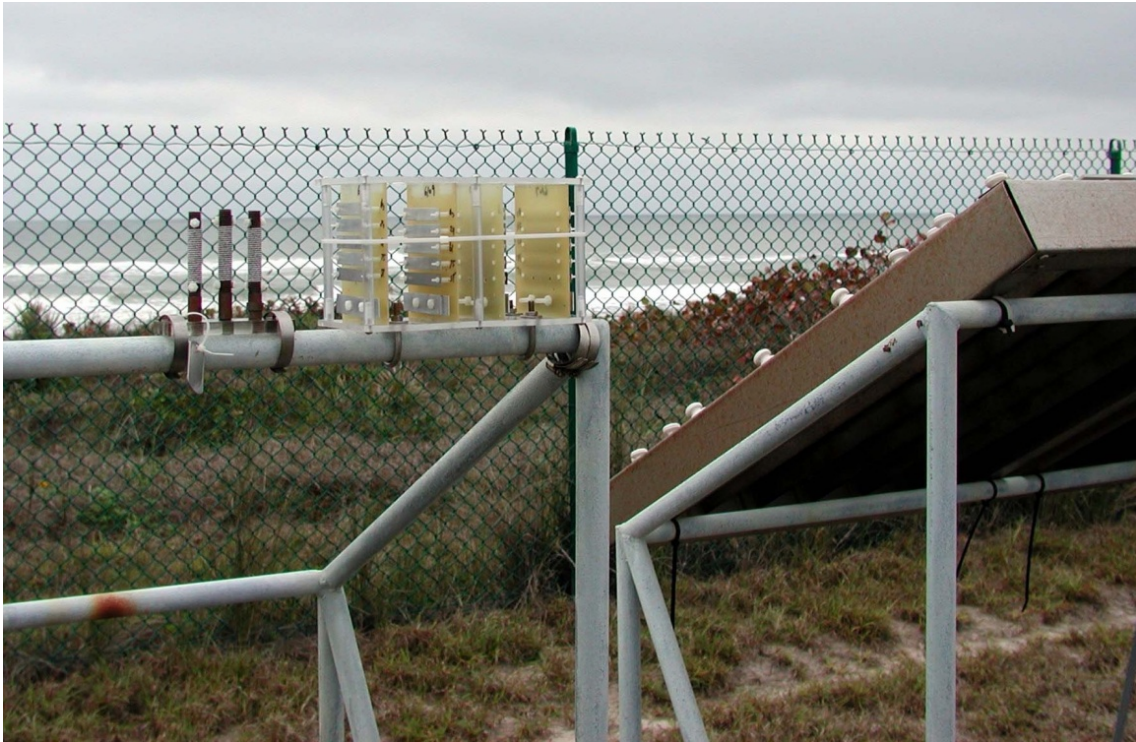
Figure 26-4: Metal Coupons in a Plastic Test Rack Exposed at the Kennedy Space Center Beach Corrosion Test Site Besides a CLIMAT Coupon (Courtesy of Battelle).
