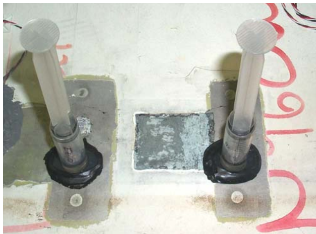
Figure 10-5: Typical Set-Up for Accelerated Exfoliation Protocol.
