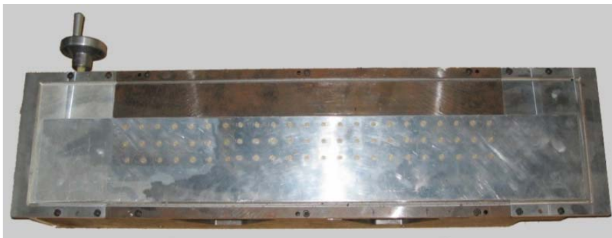
Figure 11-4: Top View of Mechanical Pillowing Simulator.
