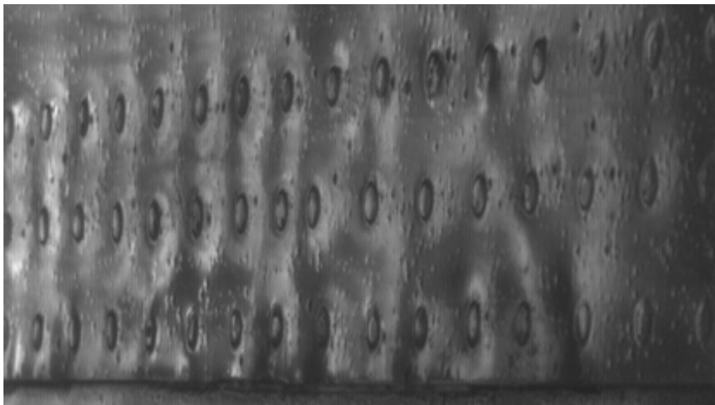
Figure 27-20: Surface Deformations from Excess Sealant in Repaired On-Aircraft Lap Joint.
