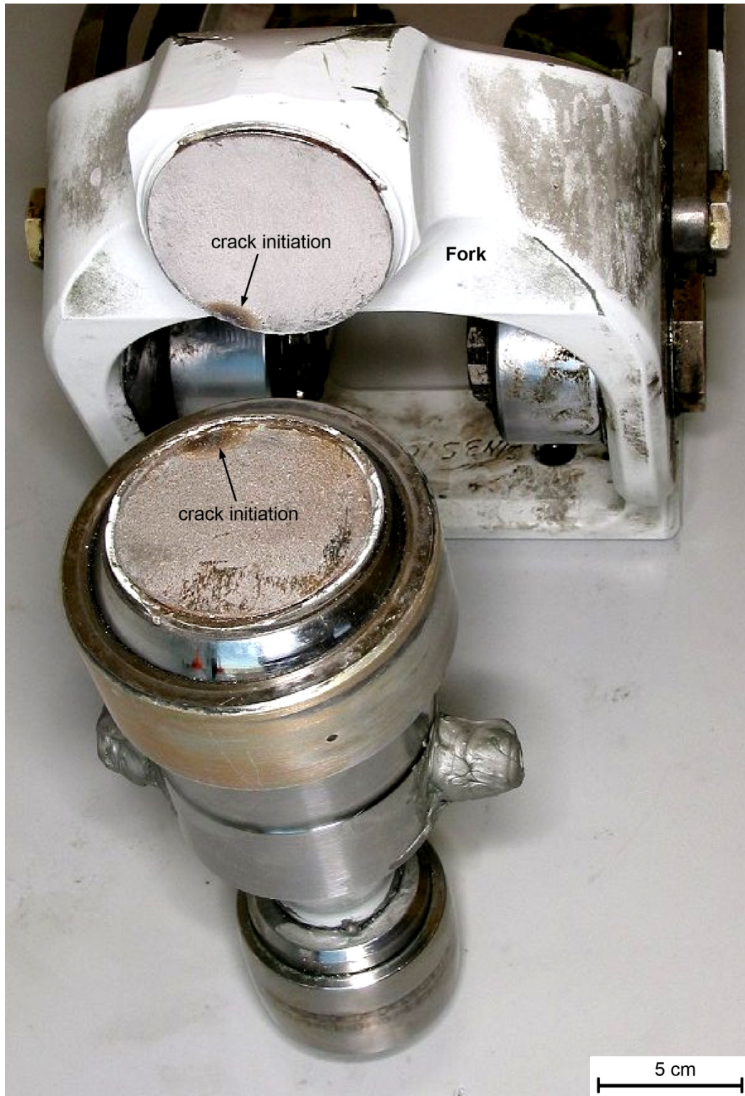
Figure 20-20: Case History 20.5.3 – Overview of the Fractured Spindle and Fork Assembly.
