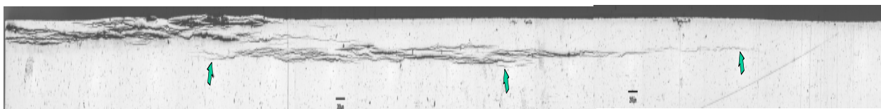
(f) Tenth polishing that removed a total of 4.902 mm (0.193 inch) from the fifth polishing.
