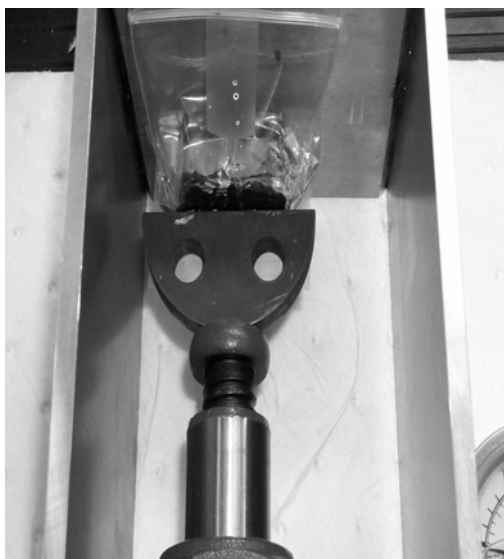
(c) Specimen placement in compression rig.
