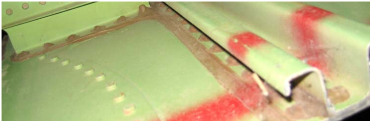
(b) View along lower surface of stringer on lap joint and body station frame attachment.
