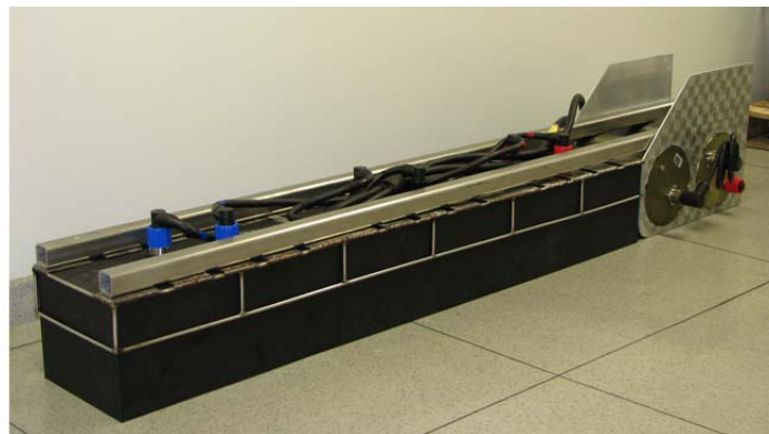
Figure 3: The Multibeam SubBottom Profiler at the stage of it first underwater test. The MSBP is currently being fitted with a nosepiece, a towing yoke, and a tail horizontal stabilizer.
