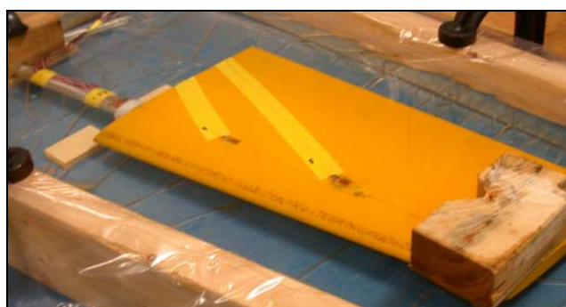
Figure 6: Static bench test of rudder strain gauges
