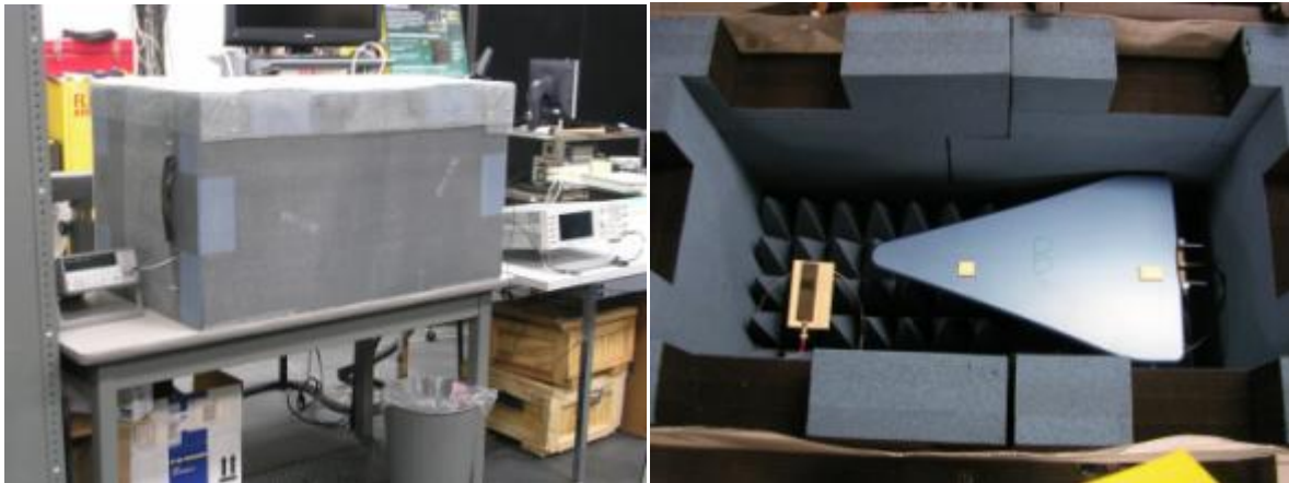
Figure 11 – Left: Anechoic chamber/Faraday cage. Right: Internal view of anechoic chamber
