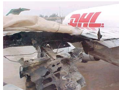
Figure 2. The Left Wing of the DHL Airbus After Suffering a SA-14 Hit. 10
