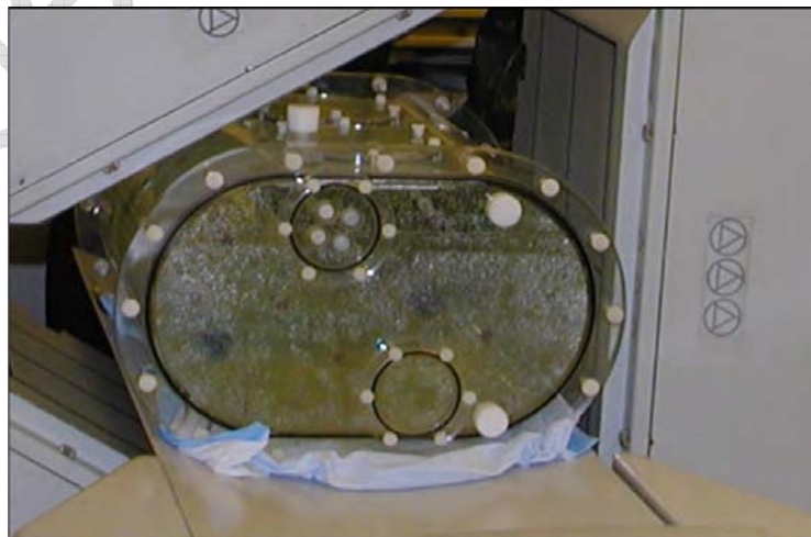
Fig. 5. The whole-body phantom was imaged by one detector on a Trionix Triad SPECT scanner using LEUR parallel-hole collimation.
