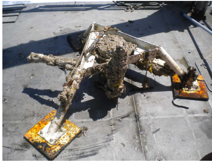
Figure 5. Recovered ADCP mooring tripod that stayed in the middle of the Nantucket Sound from December 2008 through July 2010. The SeaHorse current meter is seen attached to an aluminum arm extending to the left. Significant biofouling by barnacles is visible on all instruments.
