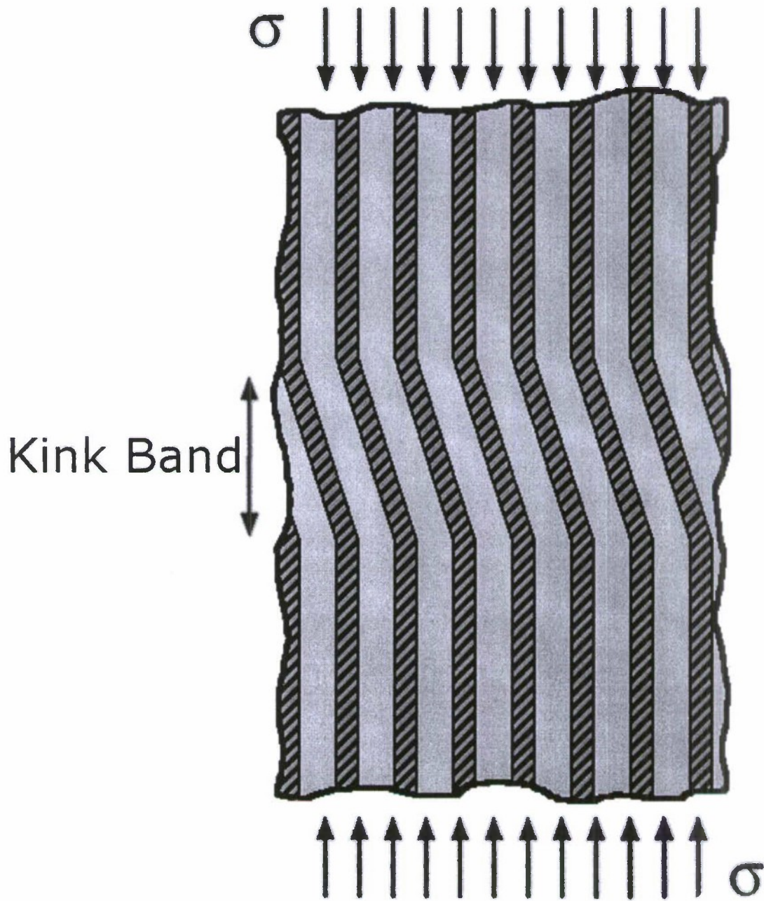
Figure 6. Illustration of plastic microbuckling and the resulting "kink band" region.
