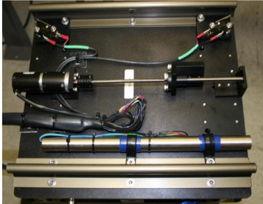
Figure 12: Top view of axis bottom plate with the gear motor, drive shaft, drive nut, limit switches, linear bearing support shafts, and position transducer
