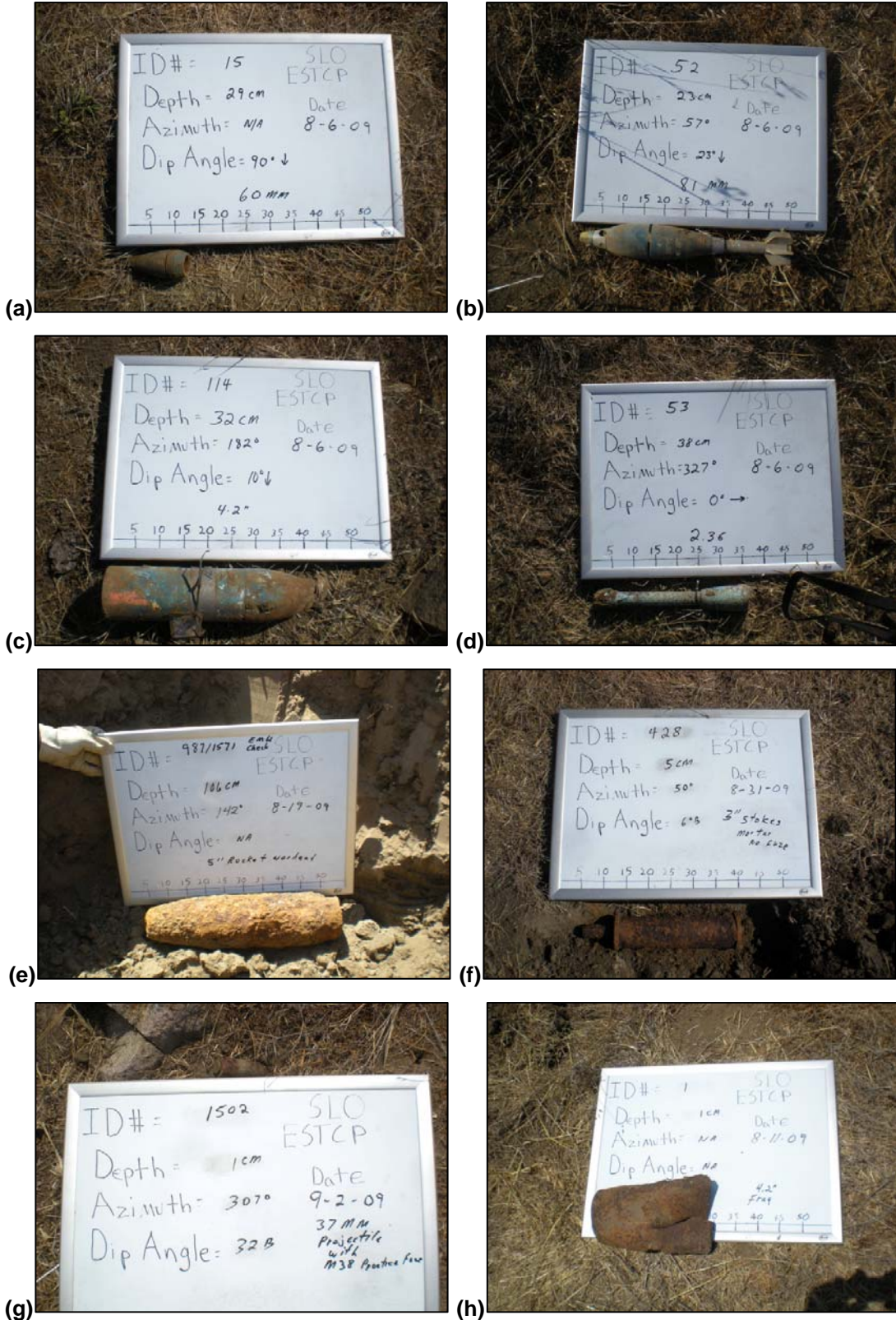
Figure 18: Photographs of recovered items, including (a) a 60 mm mortar, (b) an 81 mm mortar, (c) a 4.2 in mortar, (d) a 2.36 in rocket, (e) a 5 in rocket, (f) a 3 in Stokes mortar, (g) a 37 mm round, and (h) scrap metal from a previously exploded munition.
