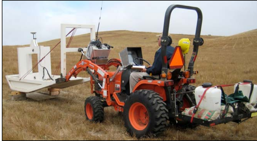
Figure 12: A photograph of the MetalMapper collecting data at Camp San Luis Obispo.
