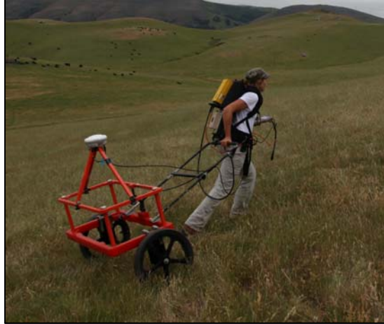
Figure 7: A photograph of the EM61 CART collecting data at Camp San Luis Obispo.
