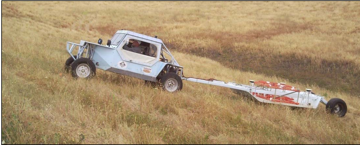
Figure 9: A photograph of the EM61 ARRAY collecting data at Camp San Luis Obispo.
