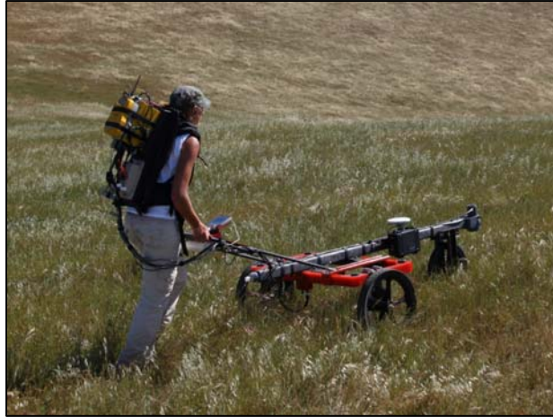
Figure 11: A photograph of the MSEM collecting data at Camp San Luis Obispo.
