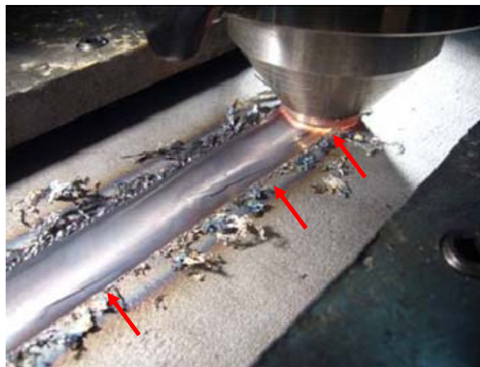
Figure 4. Shallow surface defects on the tool advancing side of dry FSW. From [13]
