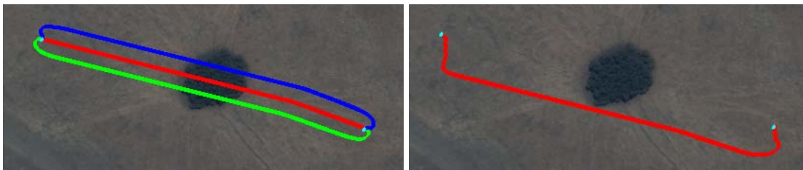
Figure 7.2: 3 unacceptable examples (left) shown along with 1 acceptable example (right). This set of examples implies 3 relative constraints (between each unacceptable example and the acceptable example); alternatively this can be viewed as a classification problem between unacceptable and acceptable paths.
