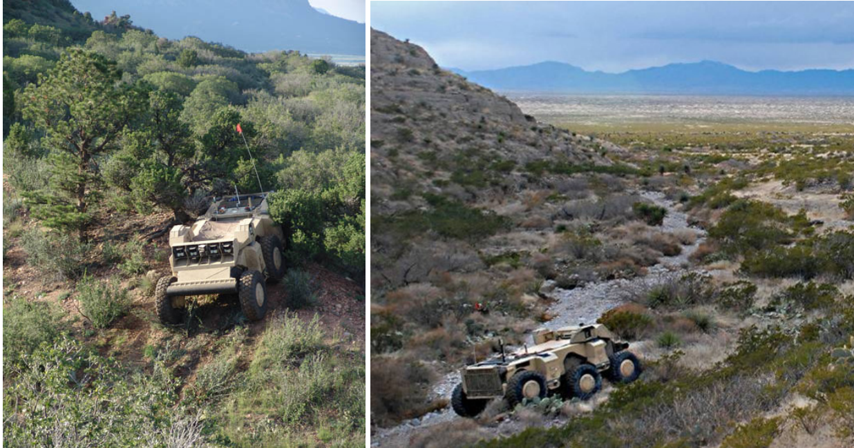
Figure 5.8: The Crusher autonomous mobile platform used in work to date. Crusher is capable of cross-country traverse through rough, complex, and unstructured terrain
