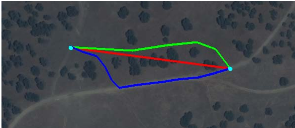
Figure 7.1: 3 Possible paths between two waypoints are shown over overhead imagery. The green path can be used as an example that is relatively better than the red path, and the blue path as one relatively better than the red and green path. Even if the blue path is not the best or most desirable path, the relative constraints that it implies can be useful for learning.
