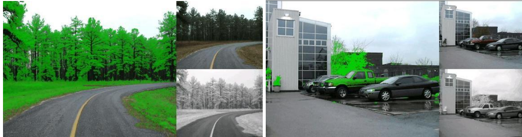
Figure 3.7: Small images show the RGB and NIR appearance of two scenes. Large images are the RGB image with areas of high NDVI highlighted in bright green. While generally reliable in natural scenes, NDVI can fail on synthetic materials such as the paint on the truck in the right image. In this case 3-D methods would easily classify the side of the truck as a rigid obstacle instead of vegetation. Note that NDVI correctly classifies the brown dead grass in the left image as vegetation.
