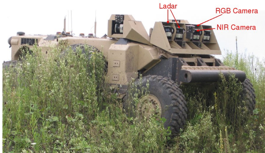
Figure 3.1: The “Crusher” robot pictured above provides state of the art autonomous driving capabilities in unstructured off-road environments, by interpreting data from onboard sensors and previously-collected overhead imagery.
