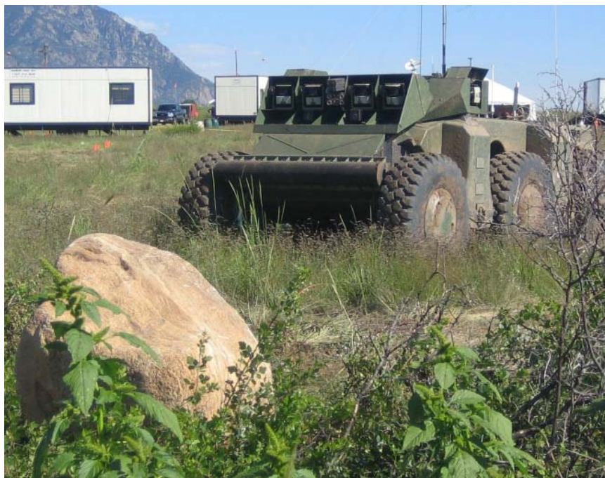
Figure 1.3: The autonomous robot “Crusher” (center), can drive through thick bushes (right) but must avoid rocks (left). Terrain classification from images is complicated by “noise” in the image from factors such as lighting weather, and camera optics.
