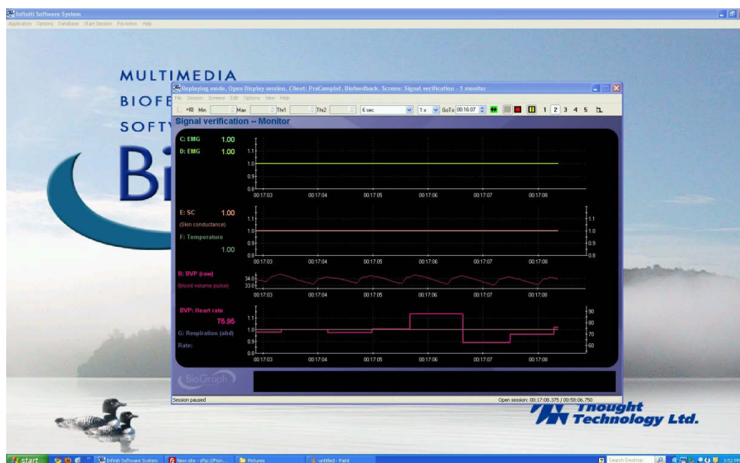
Figure 18: Multiple signal information provided by the Infiniti Software System by Thought Technology (using the FlexComp Infiniti unit). This display shows the EMG levels, the Skin Conductance, the Blood Volume Pulse and the Respiration levels.
