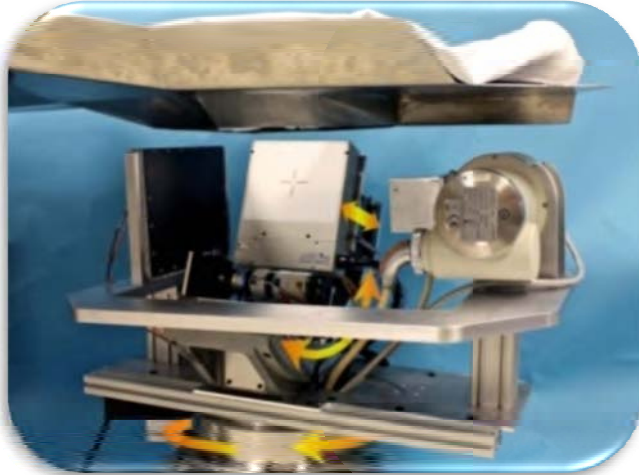
Fig. 1. Hybrid SPECT-CT breast imaging device. Orange and yellow arrows indicate the directions of movement of the SPECT camera (center). X-ray source (right) and detector (left) orbit the center-of-rotation at a fixed tilt.
