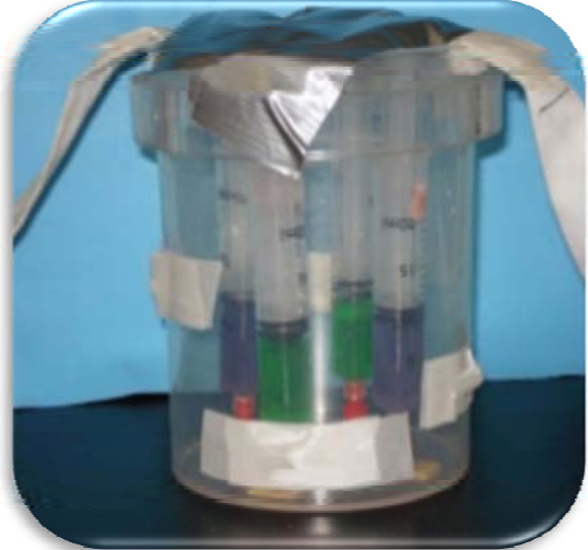
Fig. 2. Photograph of syringes with varying concentrations of radioactivity in a cylinder with an aqueous uniform radioactive background. Green syringes are filled with methanol, and purple syringes are filled with water. Medical tape attached to outside of the container secure fiducial markers used to register SPECT and CT images.
