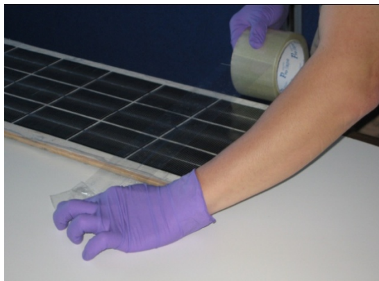
Figure 45. Solar array lamination.
