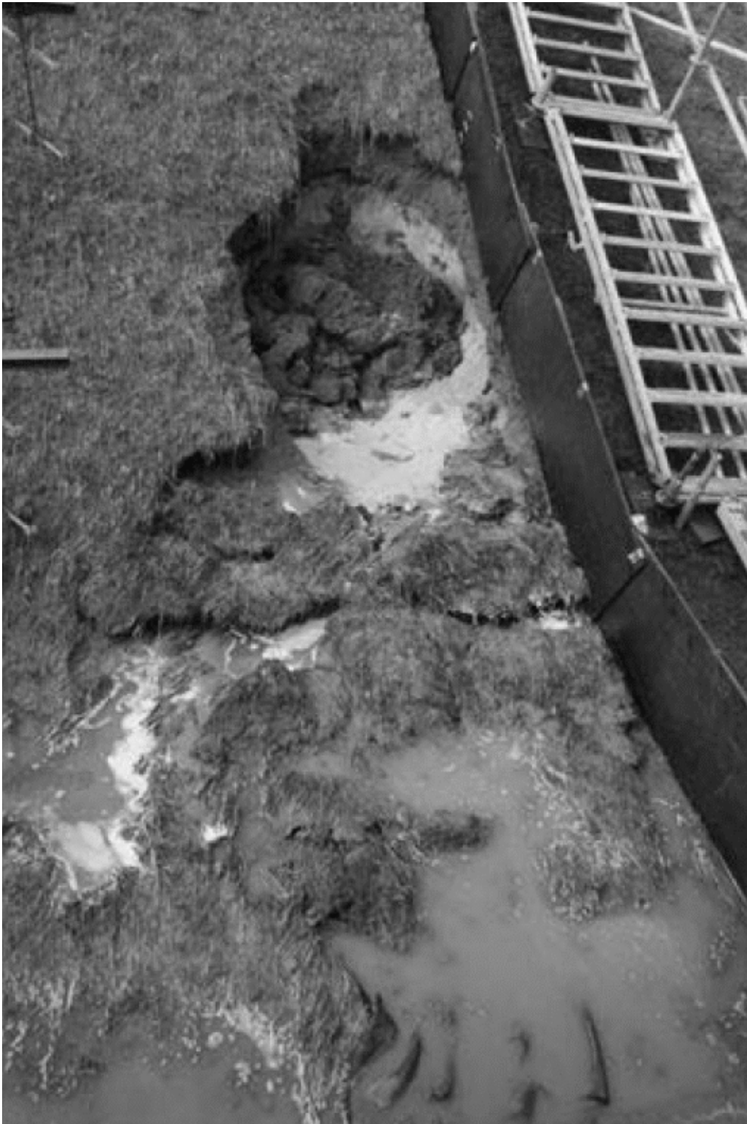
Figure 36. Slope damage at St. Philipsland after q = 50 l/s/m test (from van der Meer 2008).
