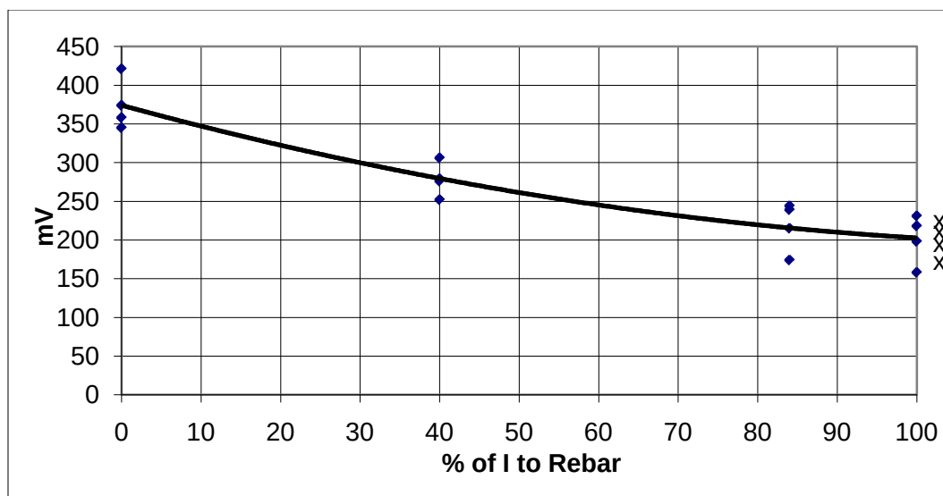
Figure E-49. Anodic shift of rebar probe when connected to EOP system negative as a function of current flow.
