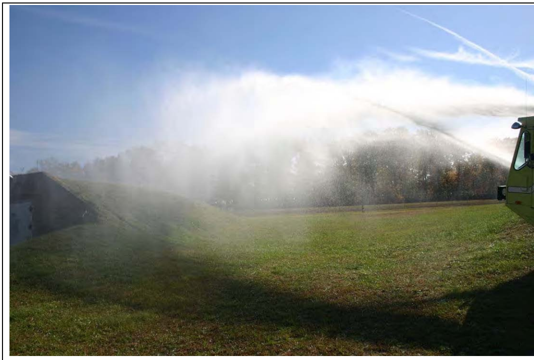
Figure E-26. Soaking of earth cover to test for leaks.
