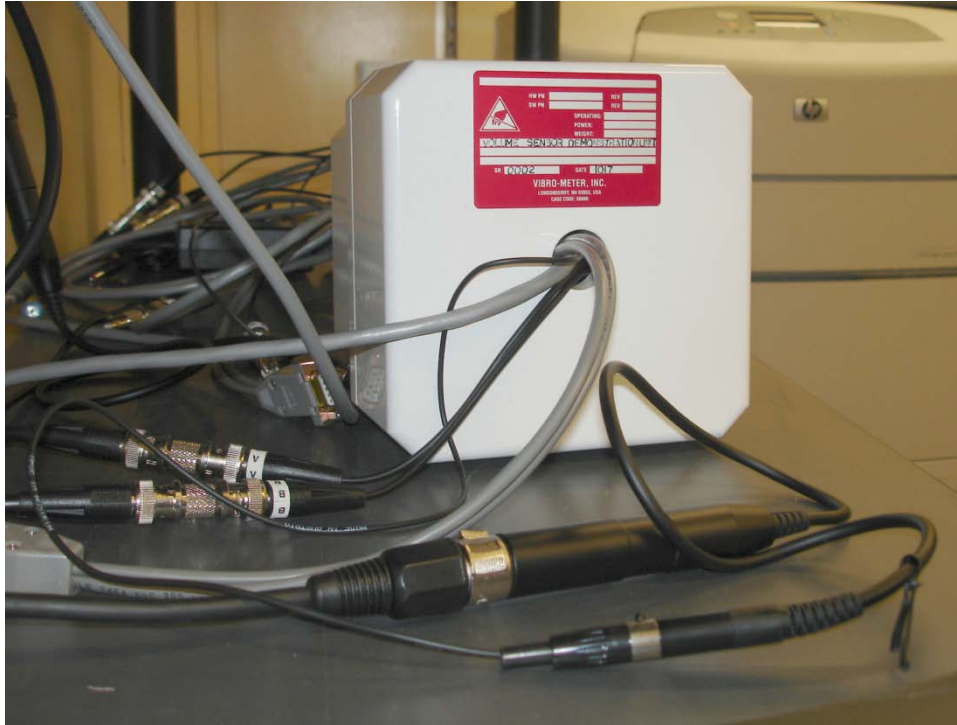
Figure 9-3 – Rear view of the Canadian Demonstrator Prototype Sensor Unit with the acoustics cables and connectors in front.
