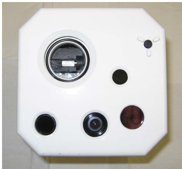
Figure 9-2 – Front view of the Canadian Demonstrator Prototype Sensor Unit with the acoustics sensor in the upper right corner.
