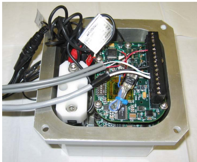
Figure 4-3 – Internal View of the Canadian Demonstrator Prototype Sensor Head
