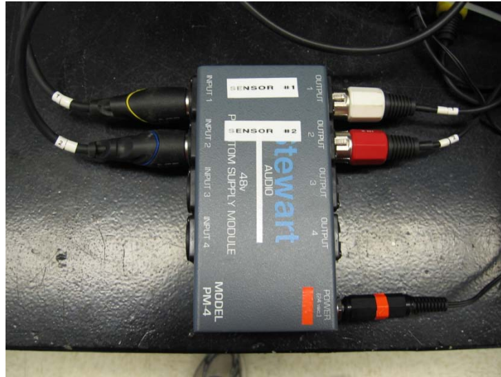
Figure 5-11 – Connections to Phantom Power Supply
