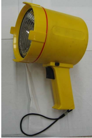
Figure 7-12 – Senseware T-229/1 UV/IR OFD test lamp
