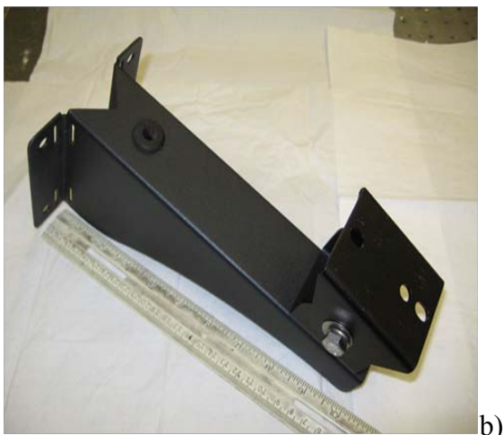
Figure 5-5 – (a) Sensor head mount, (b) SigniFire IP Camera mount
