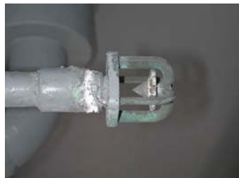
Corroded aluminum pipe at bronze CMWD nozzle
