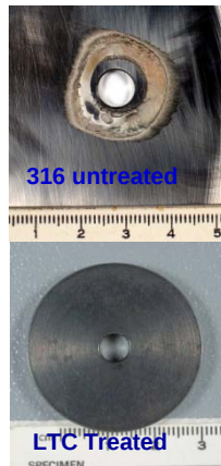
seawater crevice corrosion on 316 Stainless Steel
