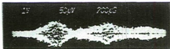
AWG signal for Shell 815 resin at 100 minutes, no visible bubbles . Saturated condition , \sim 50\mu\text{V}
