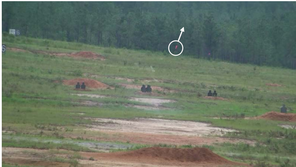
Figure 25. Same tracer round fired in Figure 24 that ricocheted after hitting ground near a 600-m target at the SA-Malone 5 range on Fort Benning, GA. Note upward trajectory of bullet.
