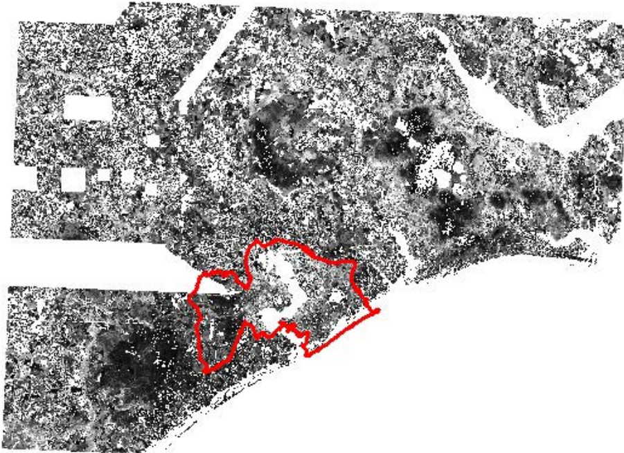
Figure 12. Canopy height DTM for all canopy height pixels > 2.0 m in height for the Camp Lejeune study area.
